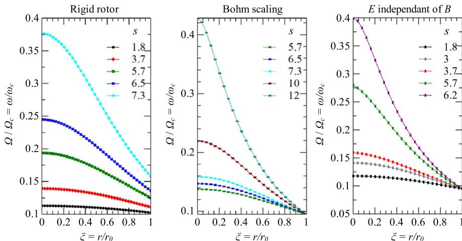
FIG. 4. Proximity to the Brillouin flow for various  $s$  values and electron-cross field regimes. The Brillouin flow regime corresponds to  $\Omega/\Omega_c(\xi) = 1/2$ . The weaker the electron cross field diffusion, the larger the electron number density required to yield a deviation from the neglected induced magnetic field case.
